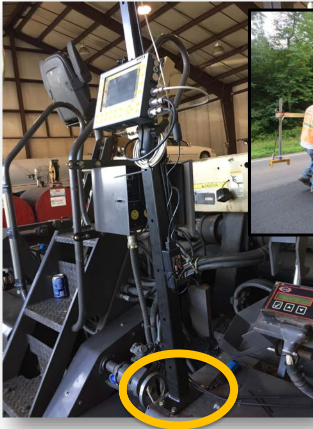
Mounted Directly to Screed
