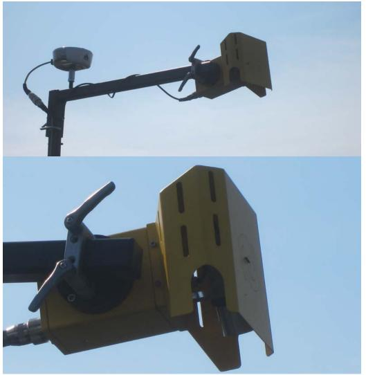
IR scan screen used to see/monitor mat temperatures in real time; attached to the mast post or extension.
