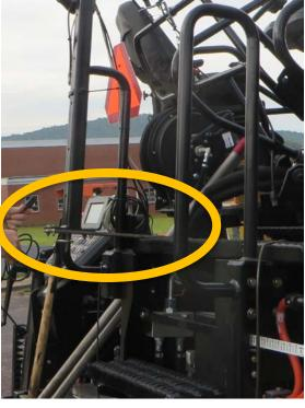
Mounted to a Steel Plate Attached to Work Platform
