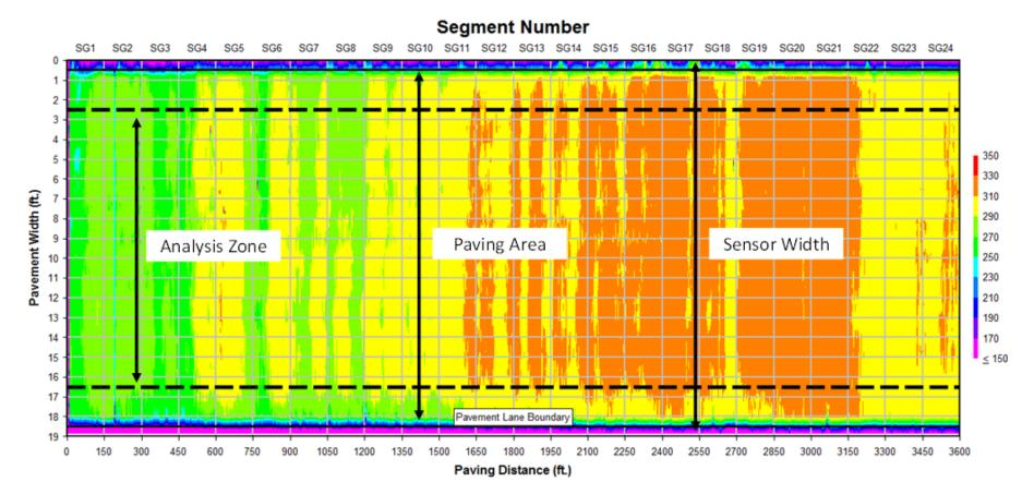
Raw Temperature Profile showing continuous improvement or more uniform mat temperatures as paving progresses.
