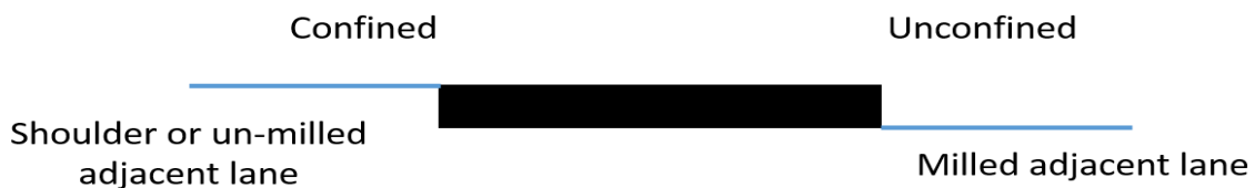
Figure 8. Definition of "Confined" and "Unconfined" Joints
