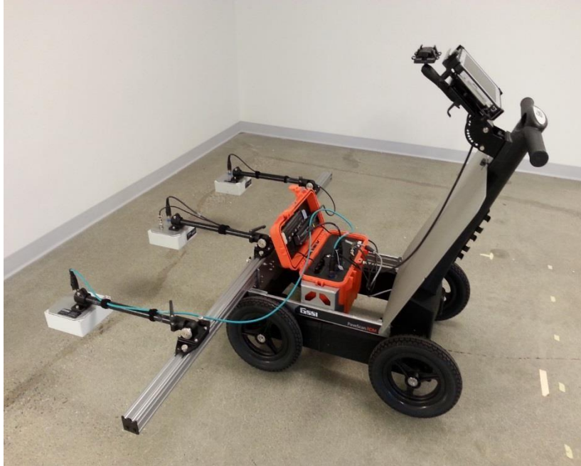
Figure 2. Side View of Rolling Density Meter Cart
