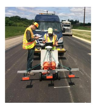
Figure 2. Three-sensor Rolling Density Meter Configuration via Extended Cart
