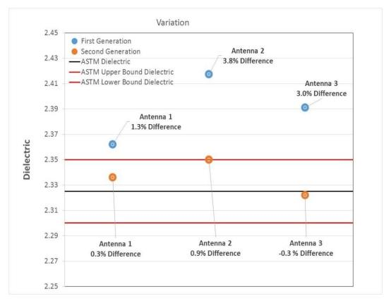
Figure 3. Short-term Dielectric Stability Measurements for Rolling Density Meter Antennas
