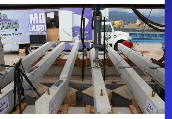
Beam Flexural Tests
