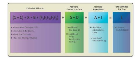
Slide Cost = 20% x Bridge Cost FX, Experience Factor FS, Site Complexity Factor FTS, Temporary Shoring Factor FJ, Vertical Jacking Factor FA, AADT/Undercrossing Factor S, Additional Site Costs D, Additional Bridge Construction Costs
