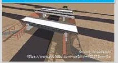
During the slide the coefficient of friction can be as low as 1% to 2%
