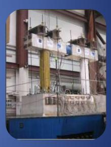
In California the focus is on seismic performance of joints connecting prefabricated elements.
