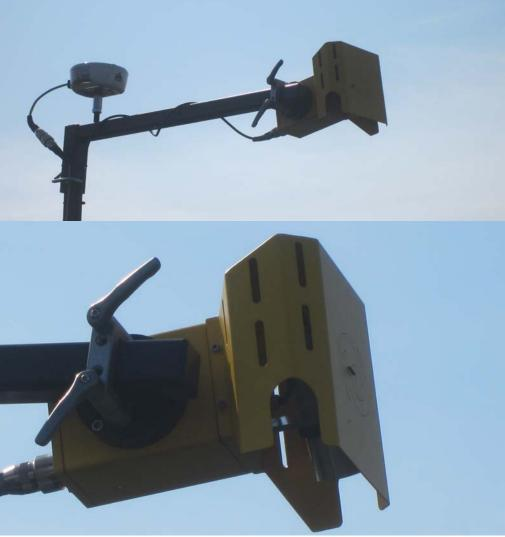
IR scan screen used to see/monitor mat temperatures in real time; attached to the mast post or extension.
