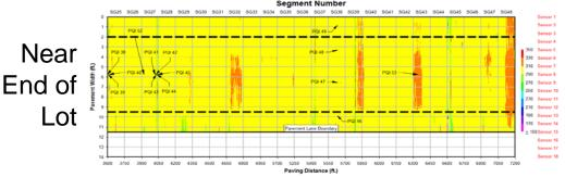
Raw Temperature Profile showing continuous improvement or more uniform mat temperatures as paving progresses.
