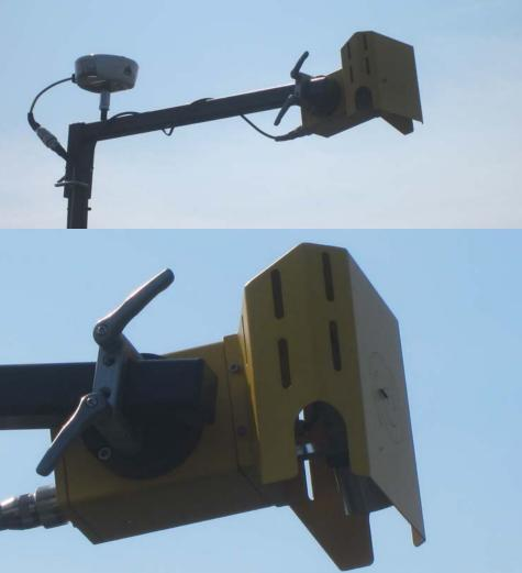
IR scan screen to monitor mat temperatures on real time basis; attached to the scanner post.
