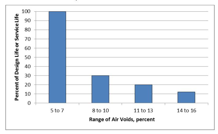
Fatigue life can be substantially reduced, as a result of lower densities because of lower mat temperatures.
