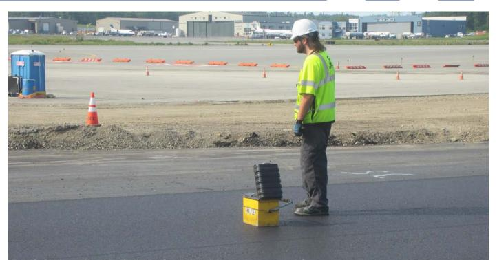
Nuclear density gauge used to measure mat density
