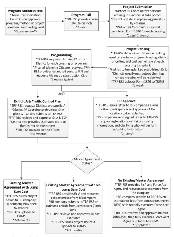
Figure 5-1. Replanking Project Flow Chart.
